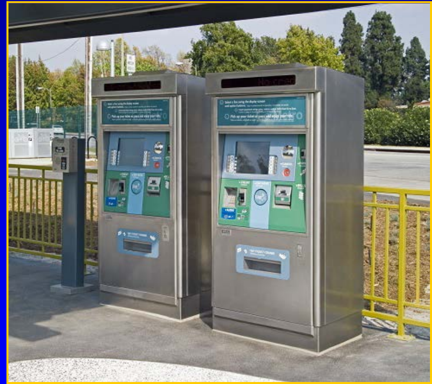
Example of TVM for Los Angeles Orange Line BRT
